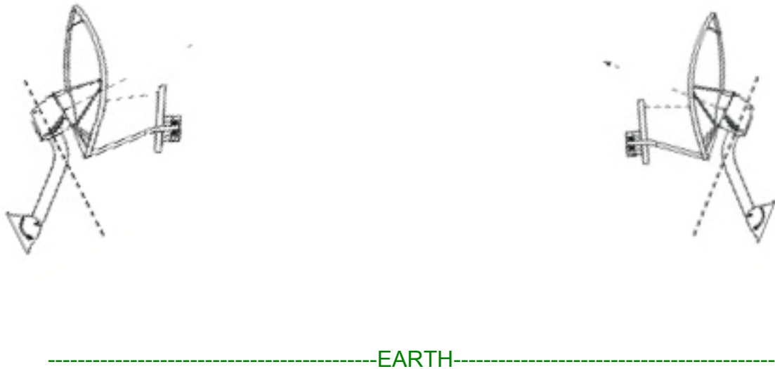
Figure 143: Incorrect mount with reflector dish
