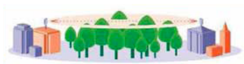
Figure 38: Fresnel zone in non-line of sight link
