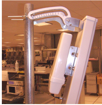
Figure 132: Down tilt adjustment bracket of OFDM AP
