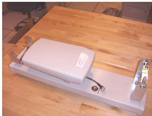
Figure 126: OFDM AP mounted to its antenna
