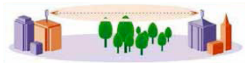
Figure 37: Fresnel zone in near line of sight link
