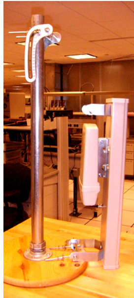
Figure 127: OFDM AP ready for tower mount
