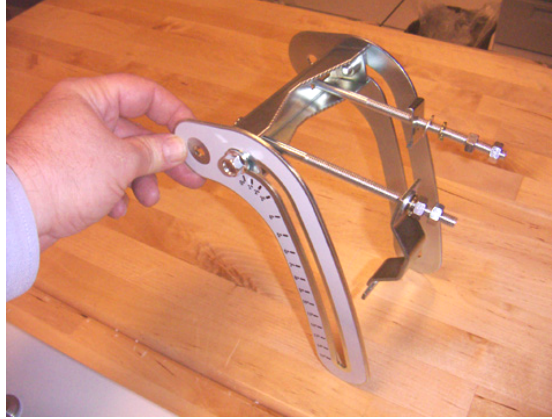
Figure 124: Assembled upper bracket for OFDM AP
