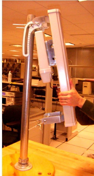
Figure 128: Hanging OFDM AP assembly onto upper bracket of pole mount
